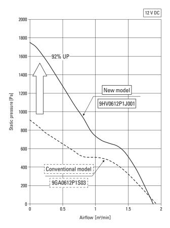
Fig. 7: Airflow - static pressure comparison
