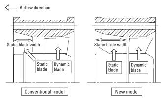
Fig. 5: Structural cross section comparison
