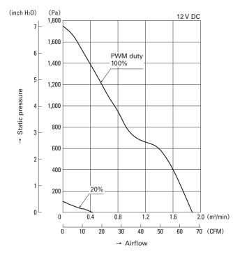
Fig. 3: Airflow – static pressure
